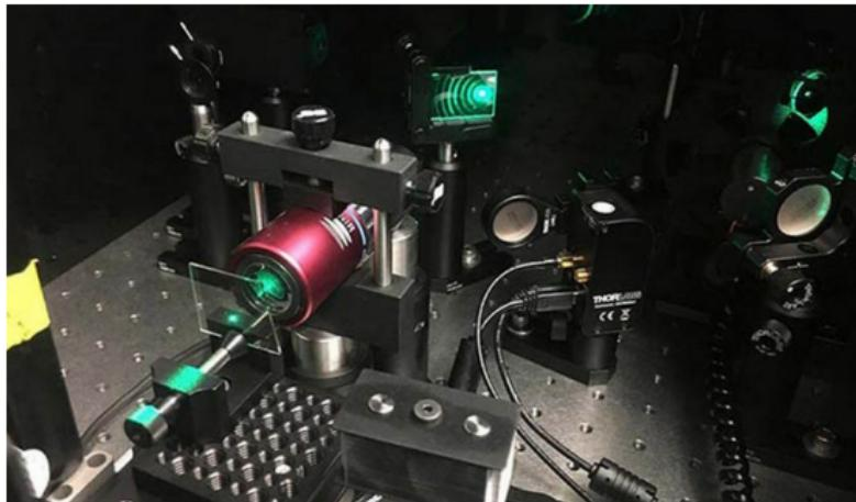
Experimental set-up of graphene production: "The preparation of a sample to be irradiated requires about **one week**." [Kotthoff, 2019]
